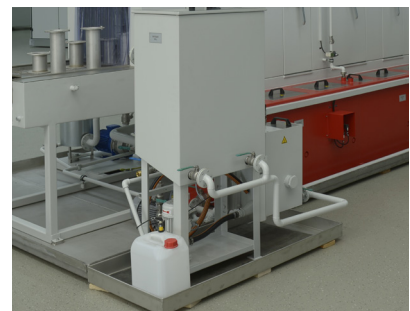
UNI oil separator – separates oils and greases floating up
