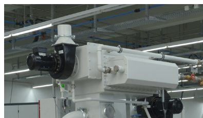
Water cooled vapour condenser (option) – extraction and condensation of the steam
