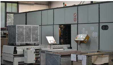
Cleaning in the mesh boxes with a payload of 1,000 kg
