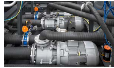
Optimised piping geometry and high pump rate for high cleanliness requirements
