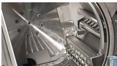
Nozzle bars with optimal spray pattern. Ultrasonic transducers in the work chamber
