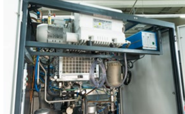
Powerful vacuum pump and ultrasonic generator if required
