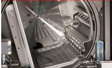
Nozzle blocks with optimal spray pattern and ultrasonic oscillators in the working chamber
